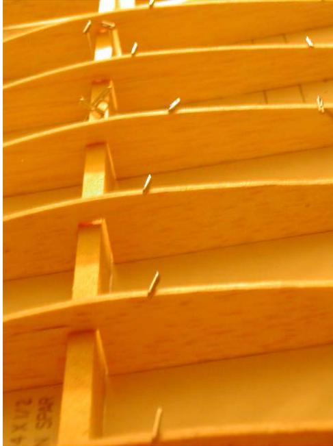
Gaps in die cutting are common problem as seen above. So what to do? One easy option is to mix up some long slow curing epoxy with micro balloons added to create a spooge. It needs to be the consistency of tooth paste. Just load up a syringe and apply in all the gaps. Make sure that you do not over do it. All the extra spooge adds weight.
