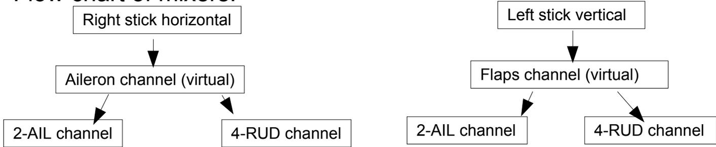
2-AIL and 4-RUD feed out to receiver aileron and rudder channels in your receiver. They are your two wing servos.
