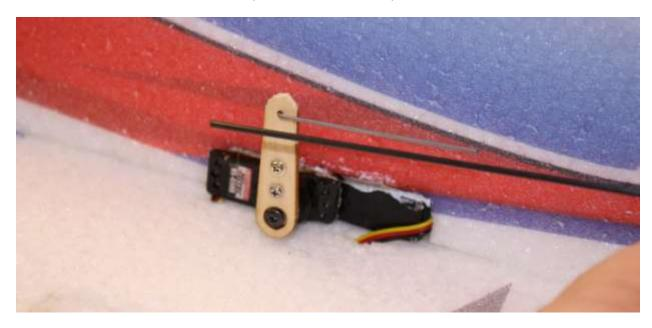
When you shrink the tubing on the servo end of the pushrods, you are working close to the foam. Use a piece of plywood to shield the foam while you shrink with a match or soldering iron.
