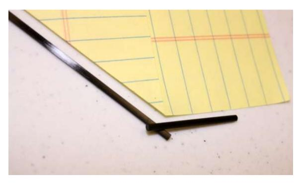
Using a drop of thick CA glue, glue the leg pieces together at the 45 degree angle. Do the same to the second set.
