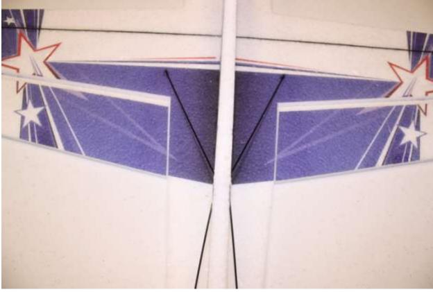
There are two more truss pieces to install in this step, they are approximately 5-6" long, however to account for variations in construction, we recommend that you measure this distance on your particular build before cutting. Install as shown.
