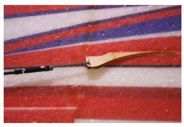
Assemble the servo ends of the pushrods. The pushrods are supplied with a bit of excess length to allow you to trim as necessary.
