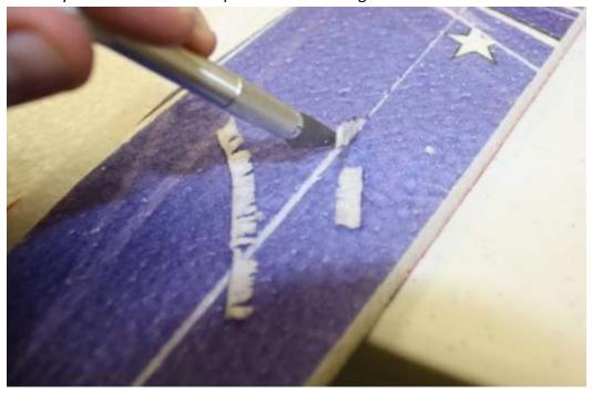
When the slots are empty, you can install the spars, starting with the pre-cut 36.5" wing spar. It is important to use plenty of welder glue for this. Coat the carbon spar in glue, and put plenty of glue in the slot. Then press the spar into the slot. Glue will squeeze out. Squeegee this glue down flat with your razor or scraper
