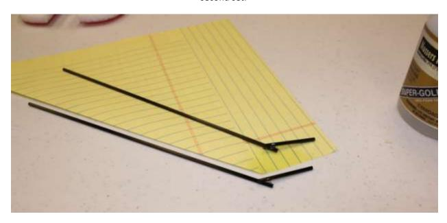
Using thick CA, glue one end of the carbon fiber yarn into the joint as shown.
