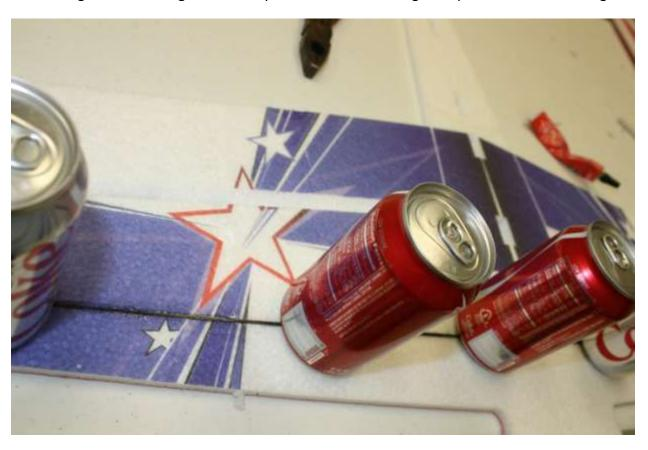
Repeat the procedure to install the pre-cut 14.5" long flat elevator spar into the elevator. Allow to dry.
