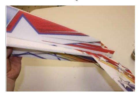
After you are satisfied with the fit, glue the upper fuselage on with Welder glue. Install the motor mount piece as well with plenty of welder glue to help align the nose, and use a drop of CA to hold the tail end perfectly together while the welder dries.
