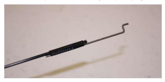
Slide the pushrod holders onto the pushrods as shown.
