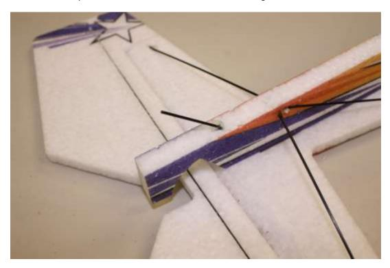
Apply a thin layer of welder glue to the nose area as shown.
