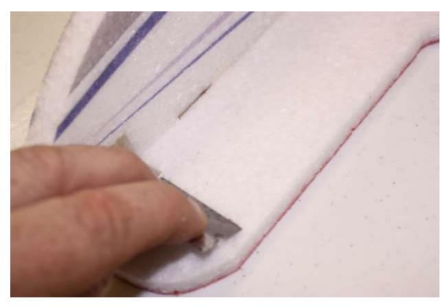
Locate the wheel pants and poke a hole with a small screwdriver as shown.
