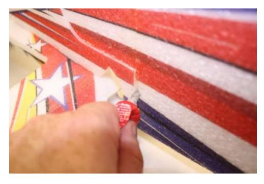
Using a hobby knife, make a pass-through slot for servo wires through the horizontal fuselage as shown.
