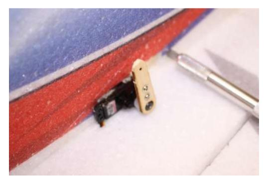
Install rudder and elevator servos as shown, if you want to preserve your servos from glue residue, you can wrap the servo body in masking tape. Use welder glue to adhere the servos.
