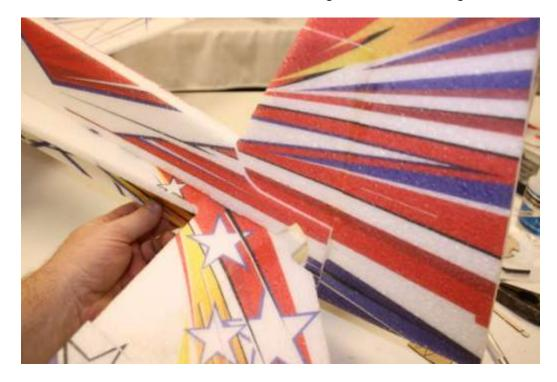
When you are satisfied with the fit, glue the vertical stabilizer to the fuselage using CA first so that if will hold alignment, and adding a bead of Welder to each side of the joint for durability.
