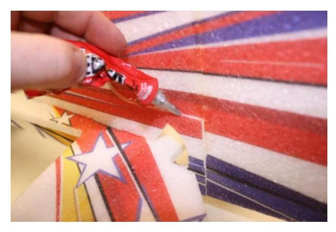
Allow to dry, then add a bead of welder glue to the bottom of the rudder which you beveled earlier. Not much welder glue is needed here to form a hinge here, wipe away excess glue and allow to dry.
