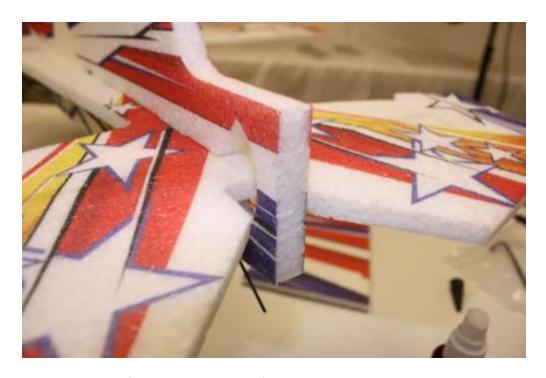
Using a sharp hobby knife, bevel the bottom of the rudder below the vertical stabilizer as shown.
