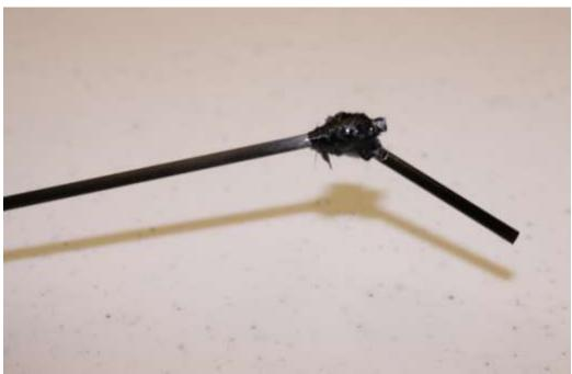
Make a cut into the vertical fuselage above the wing leading edge and insert the landing gear legs as shown. Make sure the gear legs are the same height above the wing (so that the plane will sit level when you turn it over) and tack them into place with a few drops of thick CA, then spread a generous amount of Welder glue over the spots where the gear legs meet the wing and the fuselage as shown.
