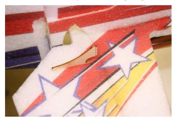
Install rudder horn into pre-cut slot as shown, using Welder glue. Trim approx3/8" from the back of the rudder horn to fit the pre-cut slot.
