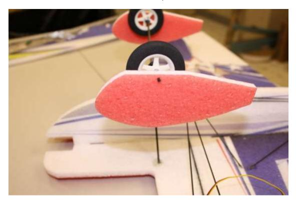
Turn the airplane right-side up to continue work. Trial-fit the upper fuselage onto the lower fuselage and wing.
