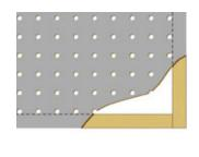
For starters, I noticed that the outermost row of holes was very close to the edge of the pegboard. If I placed this on top of the sides, the boards underneath would close off the first row of holes. This, in itself, is not a problem, but it would mean that each of those holes on all four edges would become little cups that would fill up with sawdust. So the first thing I did was to cut the pegboard right along the first row of holes. This left a 3/4" edge on all four sides.
