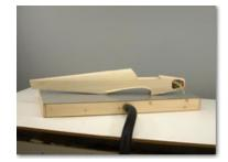
Again, being careful not to cover any holes, I glued some pieces of scrap from the sides to provide support for the center.
