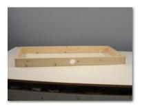
Now I needed a hole to fit my Shop-Vac hose into. With a little trial-and-error, I got the size just right for a snug fit.
