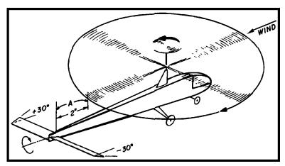
"A" must clear rotor disk. Fins may be either horizontal or vertical. As forward speed builds up, fins tend to roll fuselage to right, which induces nose-up cycling moment.
