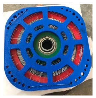
You can see in the blue plate, around the 3 through holes at each corner, I've got air vent holes, so that the poured in fill that coming next can fill around the bolts.
