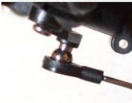
As can be seen in picture of the tail rotor ball link, one side of the connector fits best [deeper]. Just find the best supported location for the control arm ball link and push the connector down gently till it snaps in place .
