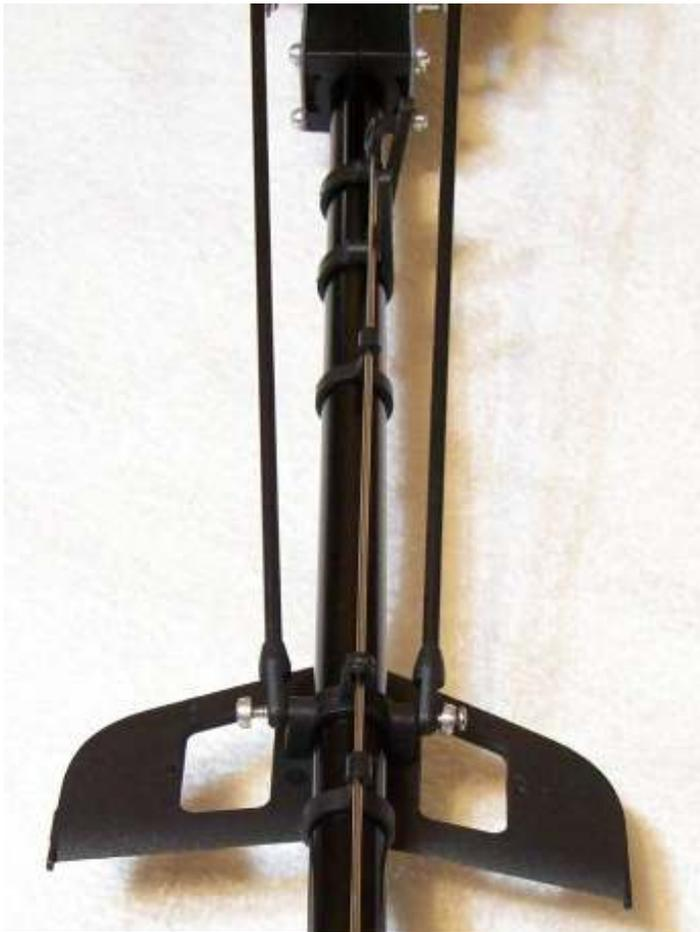
Once the tail boom braces are in place and aligned correctly. Tighten the screws and try to keep the horizontal fin at 90deg to the vertical fin or horizontally true .
