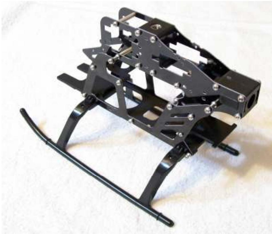
Once you have the holes in the skids matching the holes in the base of the body , you can screw the skids to the base . Next we move onto tail assembly .
