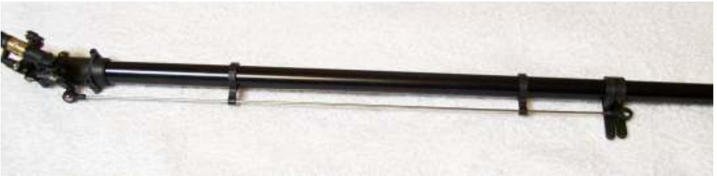
Once you are happy with the fit of the control rod , fit the tail boom servo mounts. Now your ready to install the tail back into the body of the helicopter.
