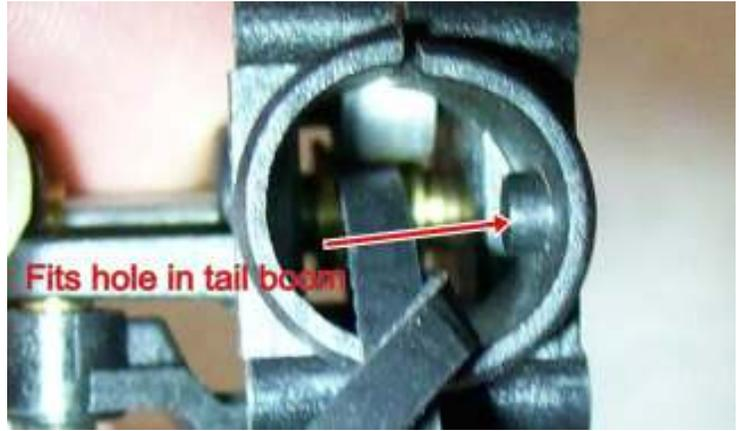
As can be seen in the picture, there is a locator built into the tail housing. This fits the hole in the tail boom. The slot in the tail boom goes into the tail boom mount in the body and it also has a locator for the slot.
