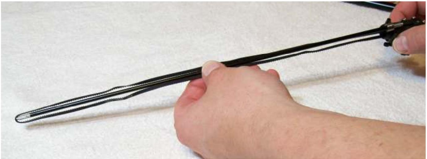
One of the more interesting tasks is getting the belt through the tail boom. I just use a rod that's not going to damage the belt to push it through the boom. Then fit the tail rotor housing correctly to the tail boom, making sure the locator fits into the hole in the tail boom.
