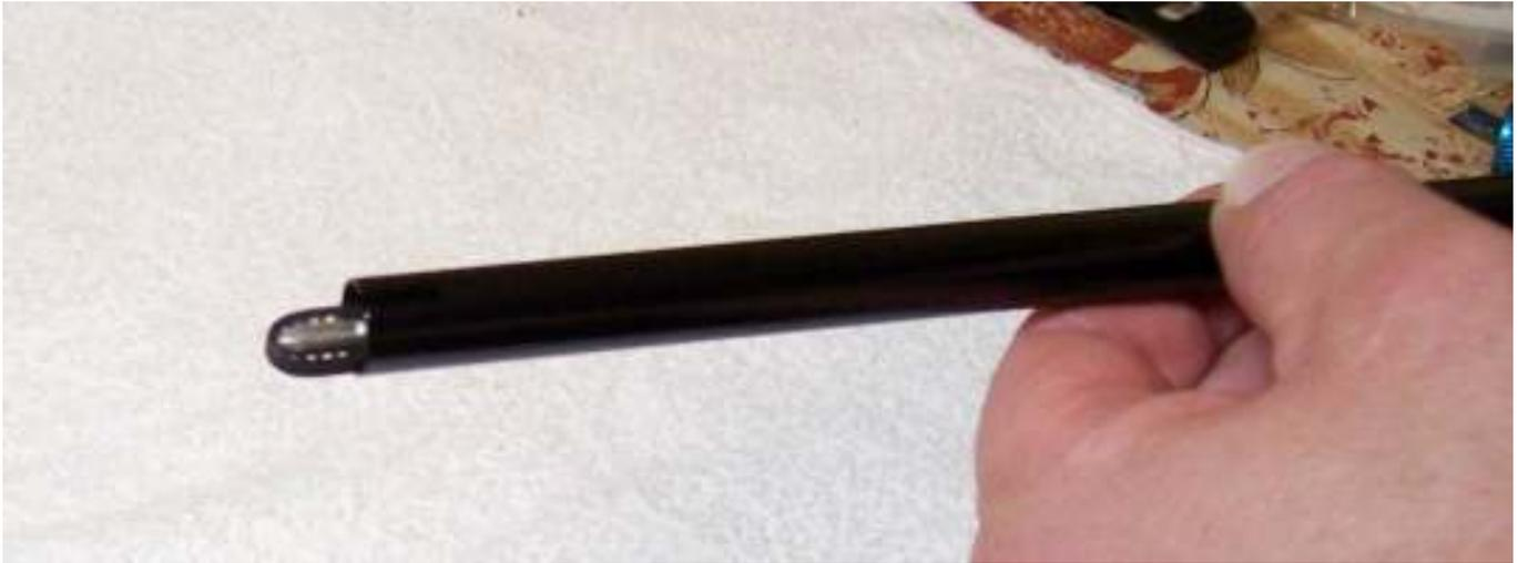
Once the belt has been threaded through the tail boom I use a flashlight to align it straight. Make sure it does not cross over itself when looped over the tail rotor drive pinion. We have to loosen some screws in the tail boom mounting block before inserting the boom.
