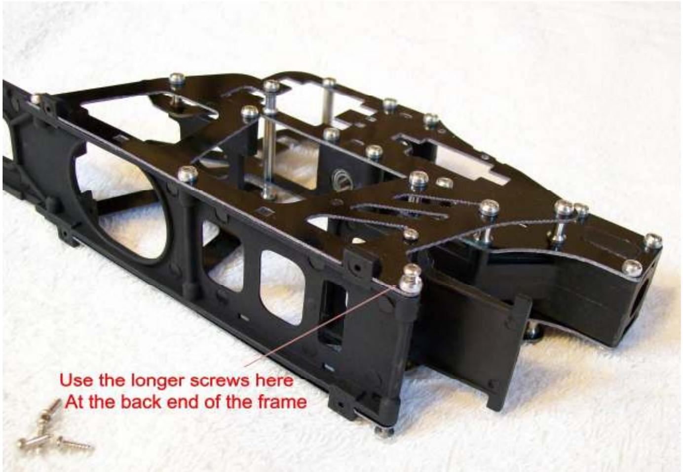
Once you get to this point it's time to add the skids to the frame. I like to put in the screws so they just protrude a little out of the other end. This way I can test fit the skids and see how the screws align with the holes in the base . If there not a good match its much easier to drill out the holes in the skids a little , so that the screws will match the holes in the base .
