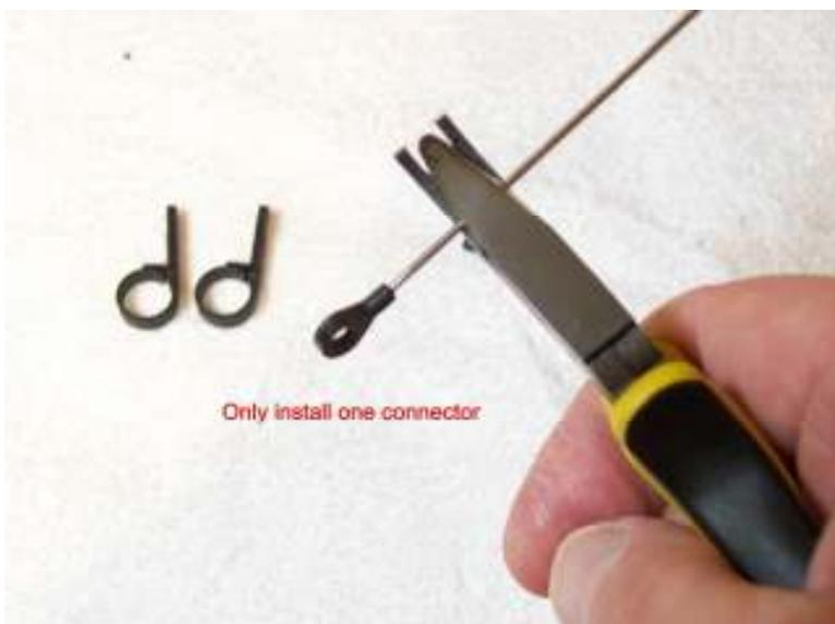
Now thread the control rod through the guides. Proceed to see which side of the ball link connector fits the ball link in the tail rotor best .
