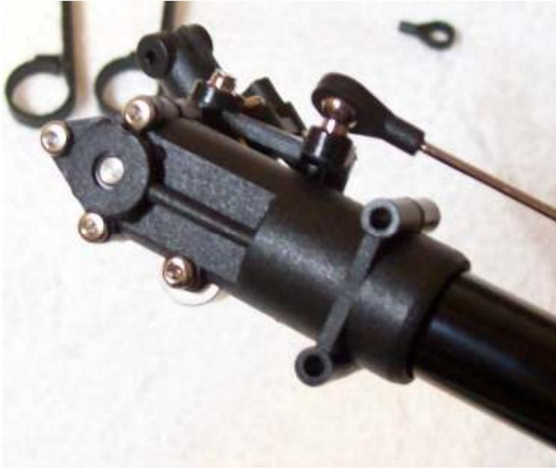
Here you can see the connector sitting in place on the ball link . Now is a good time to check for slop or binding . What you want is a nice fitting connector , not lose and not binding .
