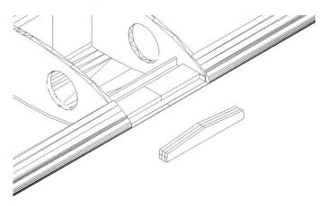
19. Locate the small plywood parts for the rear wing saddle, and assemble using thick CA glue as shown in the diagram below. Using thick CA, glue onto the bottom trailing edge of wing, between the center ribs, making sure to trim any excess covering that may prevent it from gluing properly. Measure to be certain it is centered properly. TIP: Do not use excessive amount of glue, as this piece should be able to break off in a crash, possibly preventing heavy damage to the wing.
