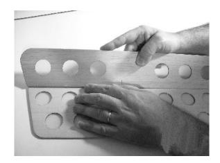
4. Turn the stabilizer assembly over, and carefully fold the elevator back onto the stabilizer.
