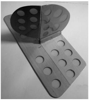
25. Attach the tail mount to the horizontal stabilizer using thin CA glue, being careful to check it is square.
