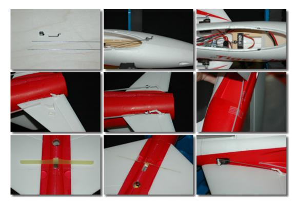
A split elevator design is used for the two halves. I like the fact that they are fully adjustable using collars as this makes it easy to trim the two halves to move in unison. The control horns work exactly as intended and snap in for ease of assembly. Once the the horns are installed and centered, the control rod tubes are taped to the side of the fuse. Not the prettiest of arrangements, but it is functional.
