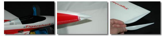
The Canopy is held on using four magnets glued to the fuse and four washers glued to the inside of the canopy. It seems to hold ok, but I would feel better if it were magnets in place of the washers. I will most likely secure with tape as an extra precaution.
