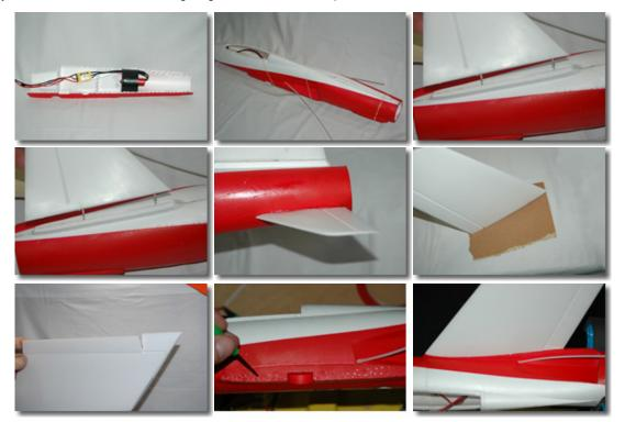
The fuse is joined together with two part epoxy. The instructions call for the fuse halves to be joined and then to join the front and rear portion together. I decided to do this is one fail swoop. I used rubber bands to hold the rear fuse halves together while I manually held the front and rear in place until the epoxy cured.
