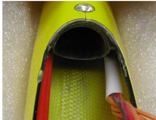
Mount the rear servo on the underside of the servo tray so that the control rods will clear each other. Dry fit everything first and position the receiver, battery, switch and servos such that the plane will balance without additional weight. When you are satisfied with the balance point, secure the servo tray with thickened epoxy being careful to avoid excess epoxy on the seams.
