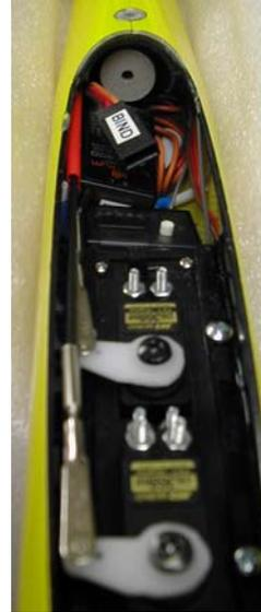
Here the tow hook has been cut with a rotary tool disk and deburred with a hand file.
