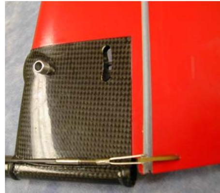
Use a rotary tool to grind out the shear webbing for control rod clearance. (Note that the supplied rods may be too short for the flaps). Solder the clevises to the rods on the servo end. The flap rods also required a bend in order to get full travel without binding. It was also necessary to extend the length of the brass control horn for the flaps by leaving a few threads exposed.
