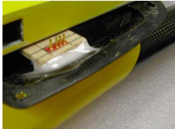
Trimming of the boom/ballast tube is optional if you require additional room for your receiver. Rough cut with a rotary tool grinder, and then smooth with an emery board or sandpaper on a popsicle stick.
