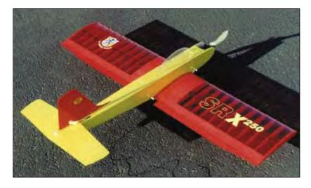
The SR Battery X250 is a low wing (36" span) Speed 400 powered electric aerobatic model. The X250 has a tricycle landing gear arrangement and the styling reminiscent of the
