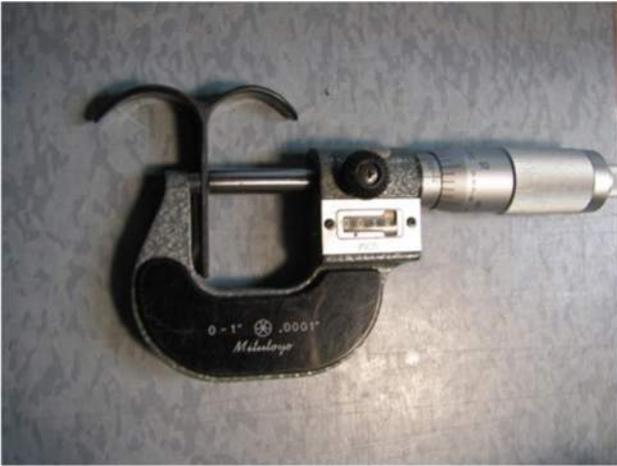
**Step 1:** Measure thickness of blade tongue.
