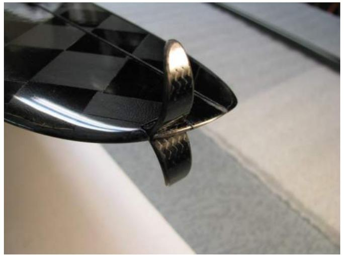
**Step 13:** Position the in-fill and glue in place with your favorite thin super glue. Due to the material lost from the saw cuts, the in-fill won't be as wide as the slot it is filling. We recommend butting it to the rear face of the slot to maximize glue contact area.
