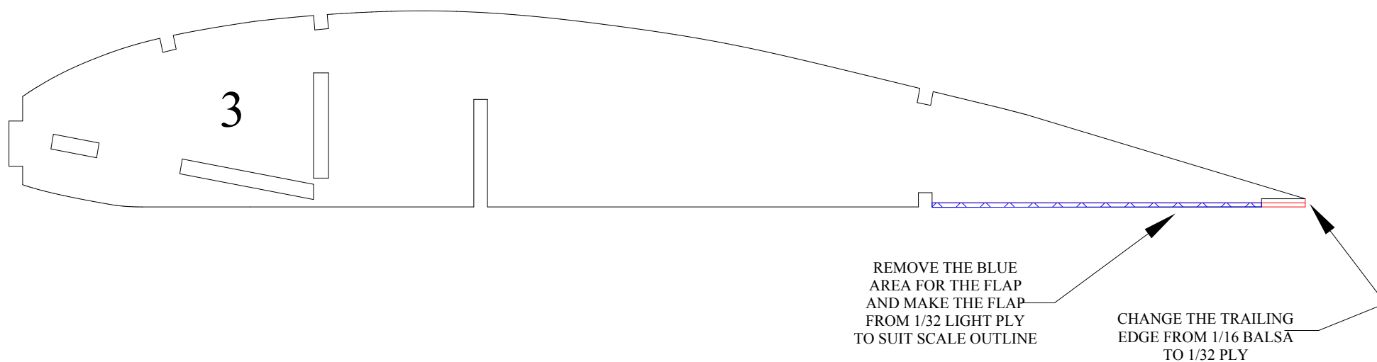
RIB 3 SHOWN WITH POSSIBLE FLAP MODIFICATION (NOT TO SCALE)
