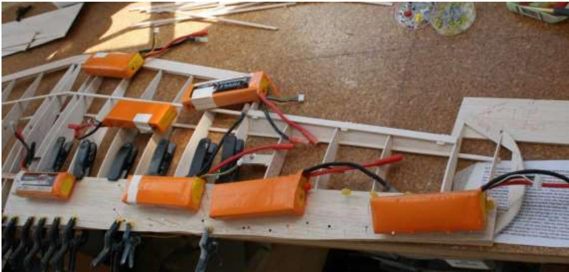
A hole was added in the centre section sheeting for the motor wires to exit upwards and at the nacelle position for the motor wires to exit downwards.
