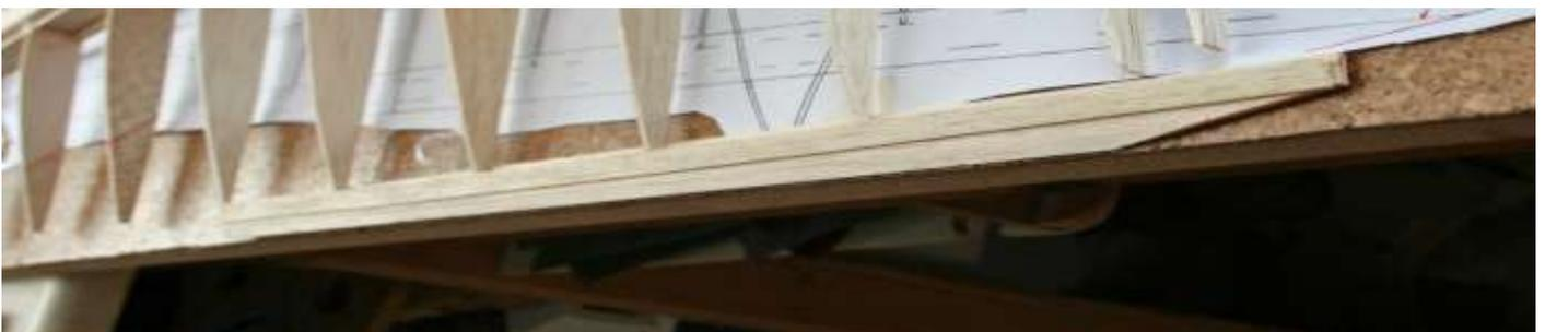
After repositioning the wing on the plan, the aileron was cut free.
