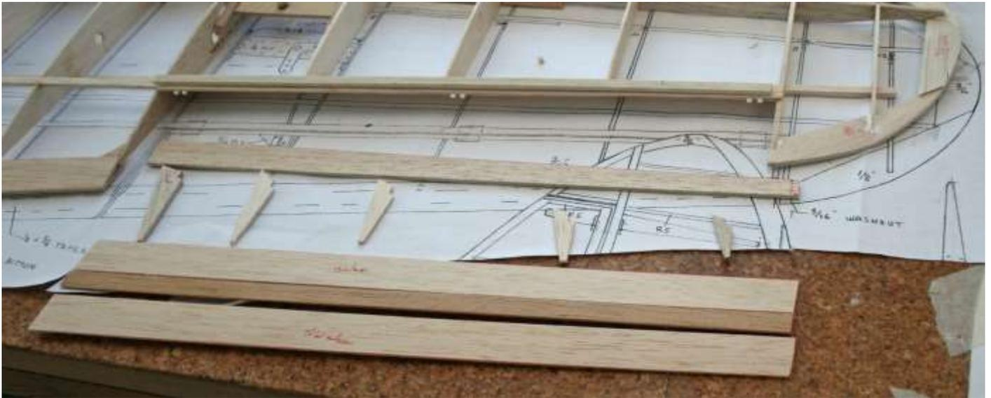
Components were then pinned over the plan with packing pieces under the front of the ribs, and glued.
