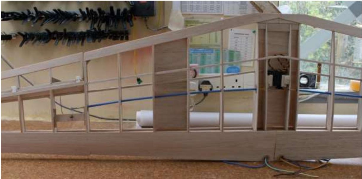
The ailerons were then fitted and hinge pins inserted. Cocktail sticks were epoxied into holes drilled through the aileron hinges to pin the hinges in place. These were then cut off and sanded flush.
