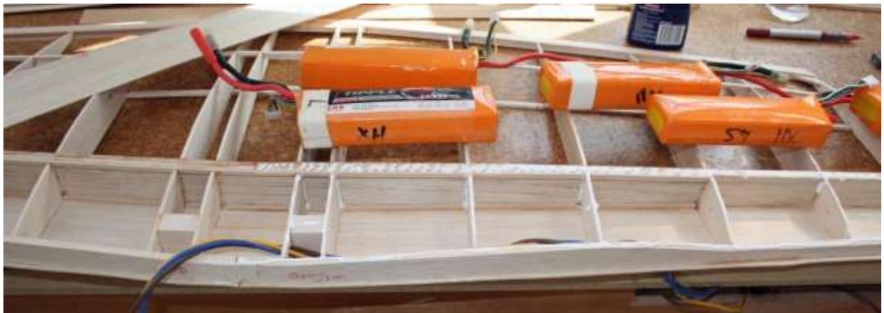
The wing was weighted down and the tip trailing edge raised to give the required washout.....
