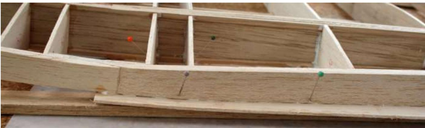
The cut in the LE sheet is seen here, allowing the sheet to follow the different curvature of adjacent ribs.
