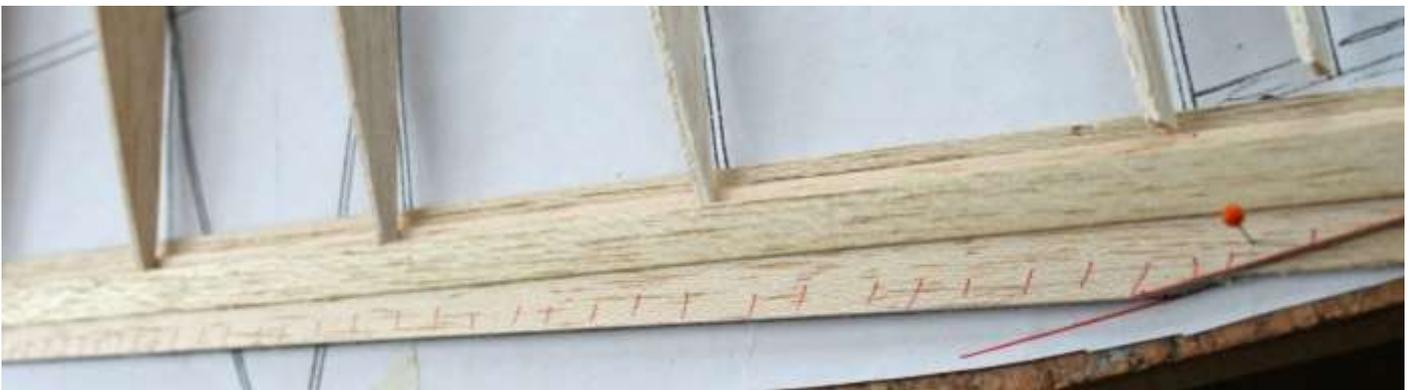
At this point it was noticed that the lower TE sheet needed to be chamfered to allow the top TE sheet to follow the curve of the ribs. This entailed the unpinning of the wing from the plan and placing it over the edge of the bench before sanding with a block.
