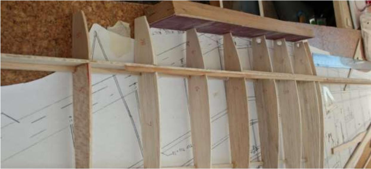
Any dimensional vagaries in the sizes of the ribs were left alone at this stage, to be sorted later with a long sanding block.
