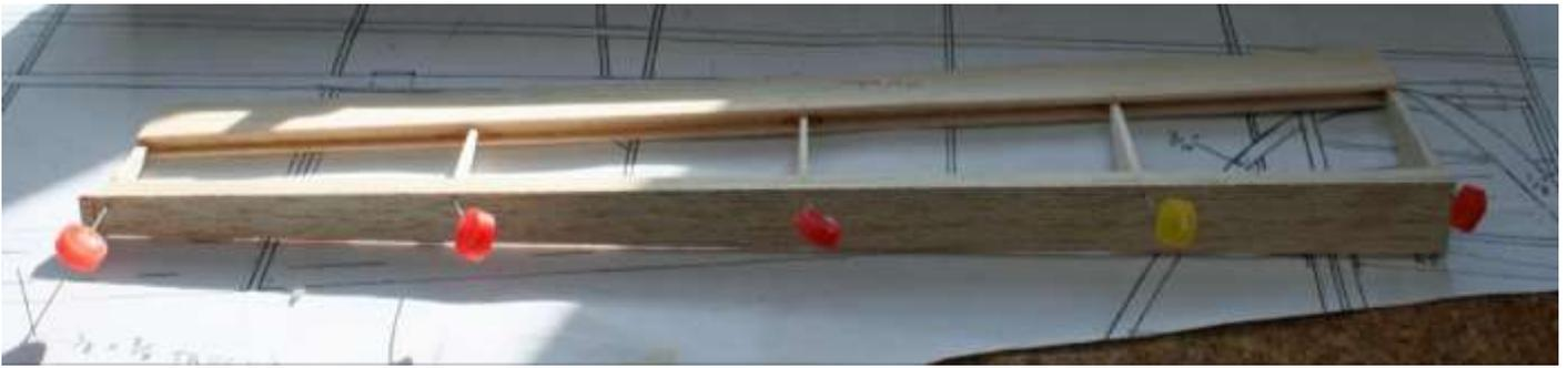
Finally the hinges were assembled, the hinge points protected from glue with a film of oil and the aileron attached with epoxy.
