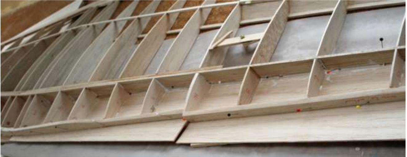
The lower LE sheet was fitted to the second wing, then three motor wires were fitted from the centre section to the nacelle positions on each side.
