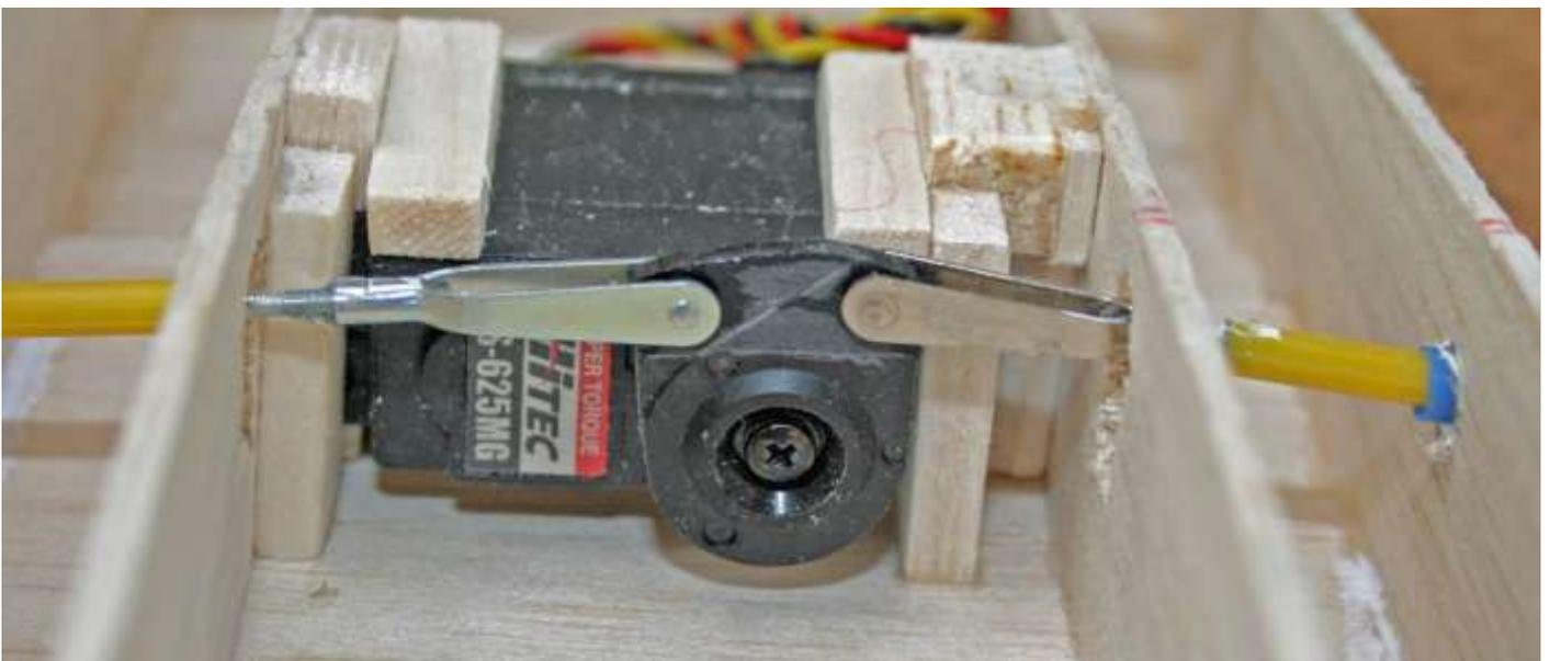
Snakes were fitted in position, using squares of 0.4 mm ply at each rib to support the snake outer. Each snake outer was bonded to two of the ribs, using epoxy.
