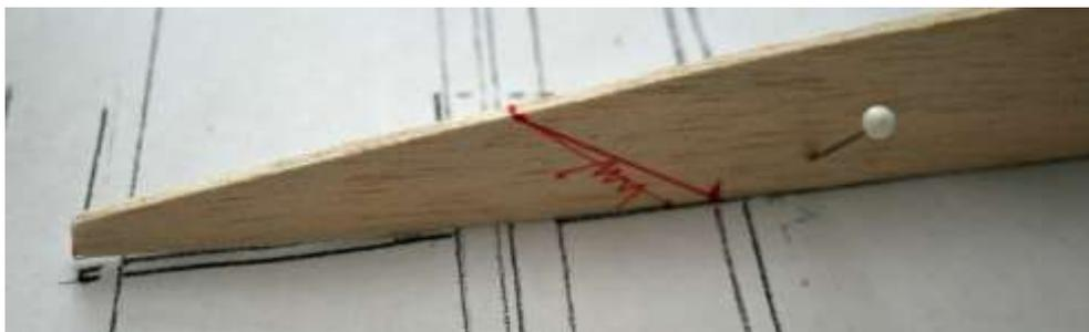
The upper and lower trailing edge (TE) components for both wings were cut out from sheet balsa. Stock trailing edge section was cut down to make the 1/8 x 3/8 tapered insert.
