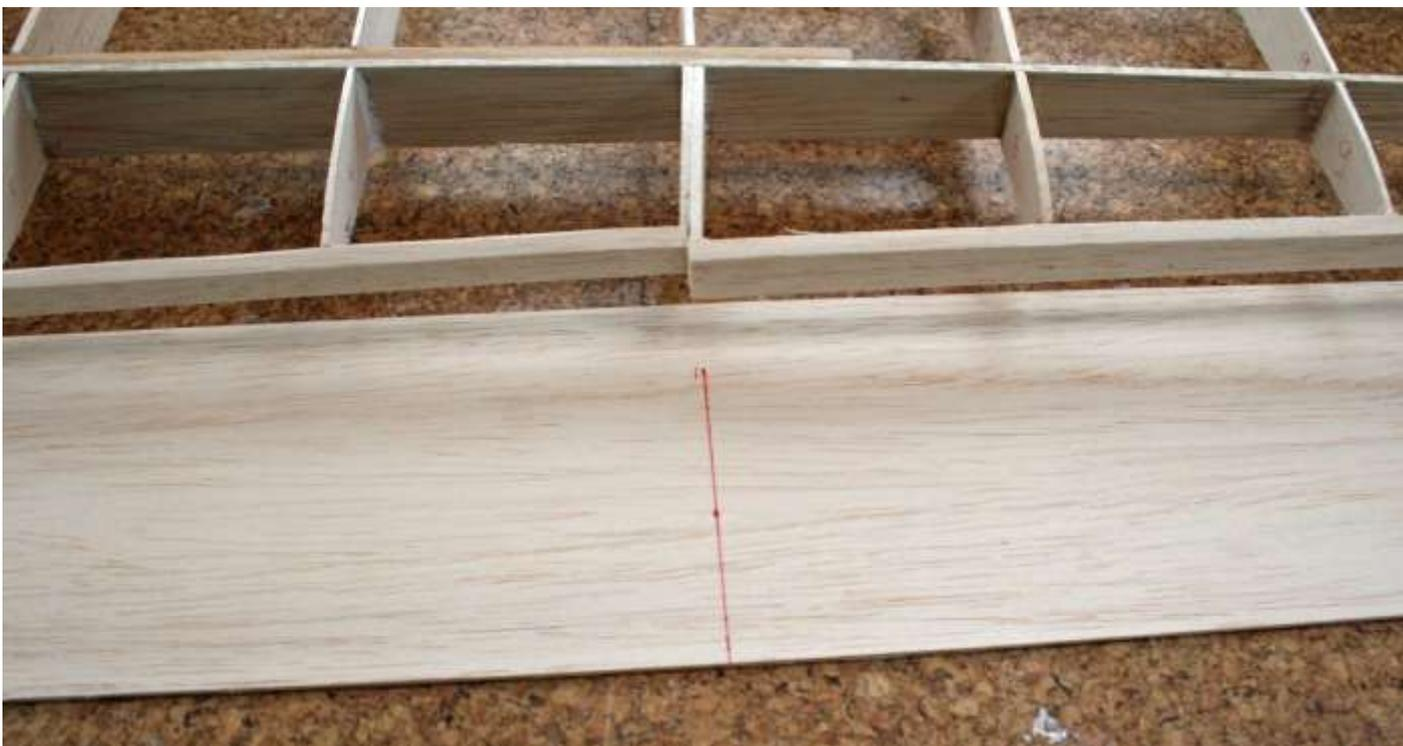
The LE sheeting was attached using PVA glue, with occasional tacks of cyano to hold it in place while drying. TE section stock from the spares box was used to support the sheet under the LE.
