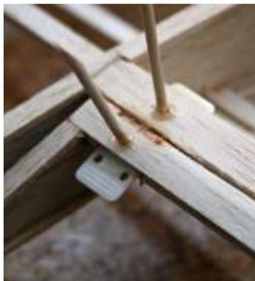
The shaped strip under the aileron hinge line was made up from triangular strip and glued in place. Clearance with the aileron was checked over the full aileron movement.
