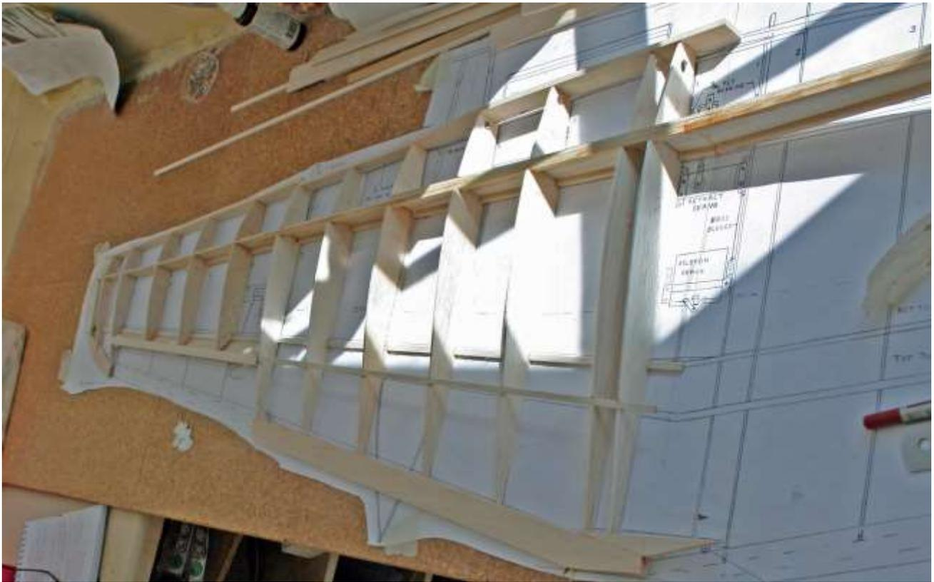
Aileron hinges were then inset into the top spar, aligned with piano wire and straight edge and epoxied in position.
