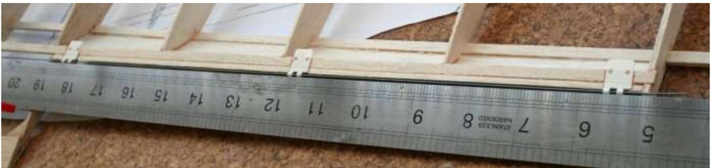
The inner leading edge (LE) sheet was then shaped and fitted. Note the difference in height between the wing inboard and outboard of the nacelle position. Also note the step where the NACA cuff starts.
