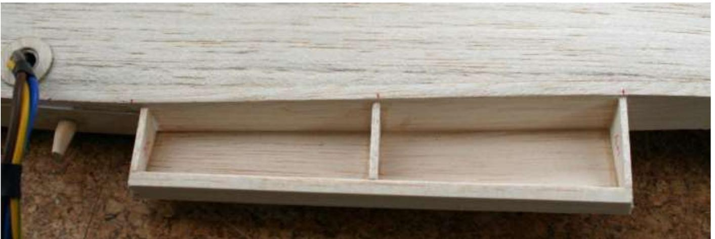
...followed by the top sheet and outer leading edge. The outer leading edge was made from LE stock.
