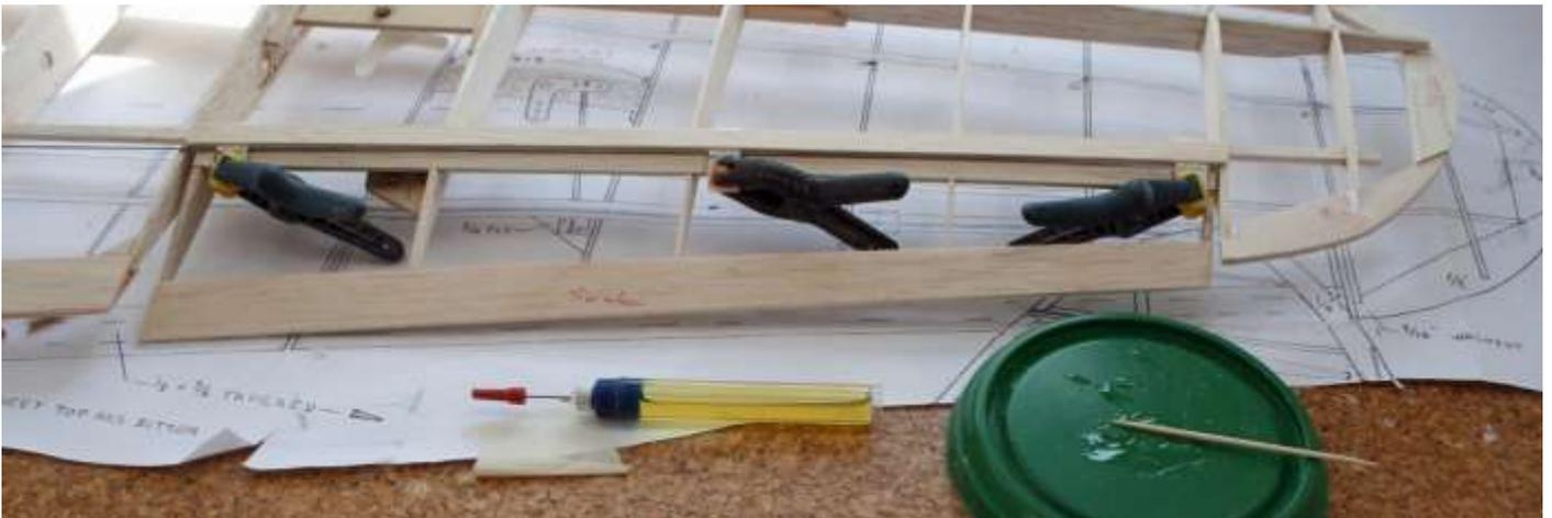
When the epoxy had set, the aileron hinge pins were withdrawn and the aileron removed to a safe place.
