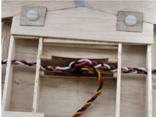
The fixed plug in the fuselage is epoxied onto a piece of liteply fitted to a servo rail and existing balsa cross-piece.
