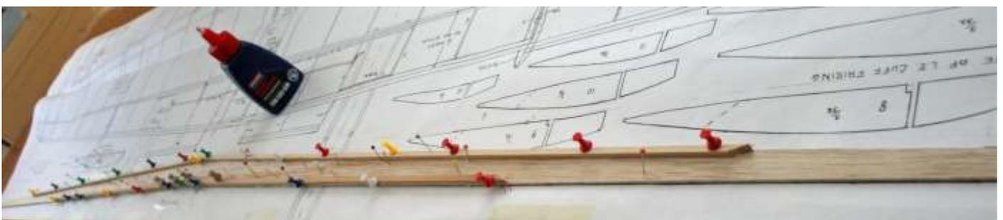
The spar was lightly sanded top and bottom to remove any extruded glue from the joints, before it was pinned it vertically over the plan ready for attaching the ribs.
