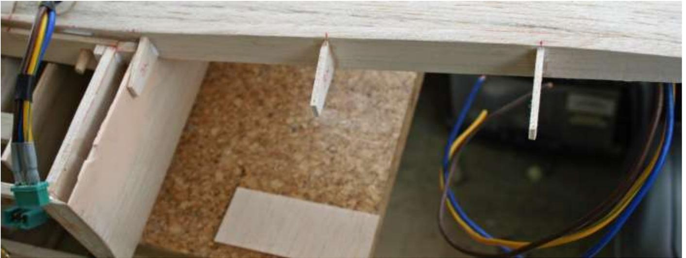
The wing was removed from the fuselage and the inner leading edge and lower sheeting fitted.....
