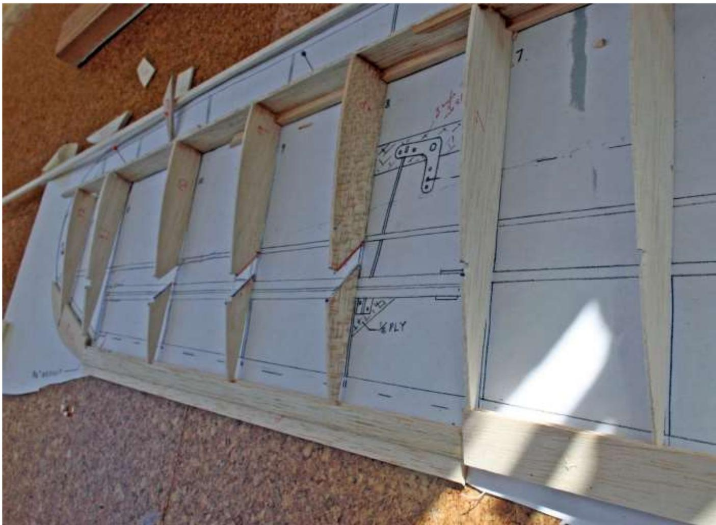
The sub spars were then added, followed by the sheet at the aileron cut-out. The depth of cut for the sub-spar slots was marked onto a razor saw using masking tape, to make accurate cutting easier.
