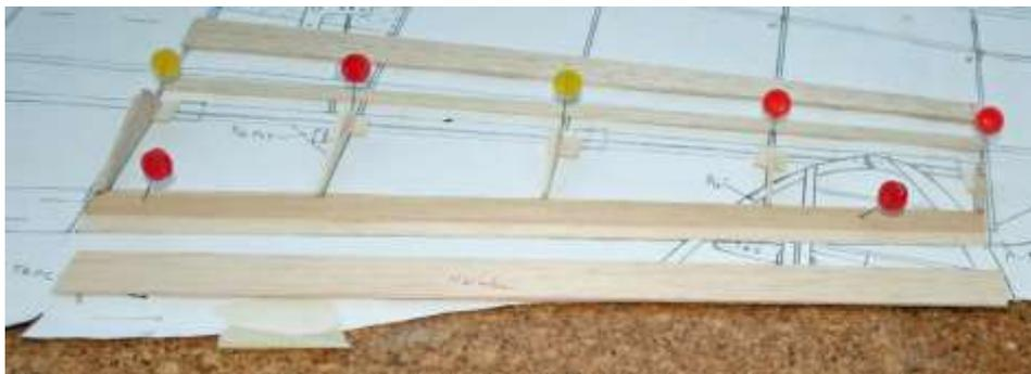
A top strip (not shown on the plan) was added to match the sub-spar on the wing to make hinge attachment easier.
