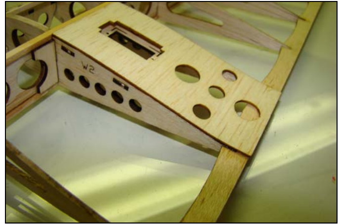
19. Flip the wing over and glue the cover to the inside. Sand cover flush with trailing edge.
