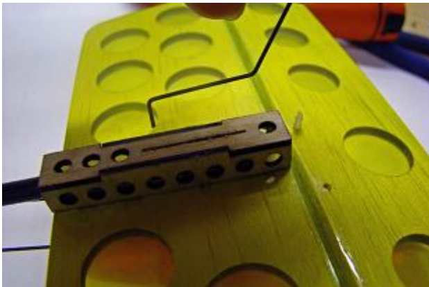
Install tail skid into the tail support bracket
