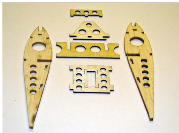
Center ribs W2, servo deck P10, front wing saddle P11, P9 and main spar brace
