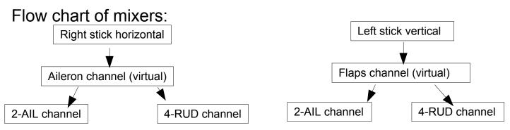
2-AIL and 4-RUD feed out to receiver aileron and rudder channels in your receiver. They are your two wing servos.
