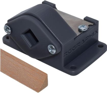
Thank you for your interest in the RG Graphix Balsa Tri-Stock Stripper. This handy tool features a heavy duty blade and comes with three standard adapters- 1/4", 5/16 & 3/8". With these three adapters 1/8", 5/32", 3/16", 1/4", 5/16" & 3/8" triangle stock can be produced. And with the optional 1/2" adapter, 1/2" triangle stock can be made.
