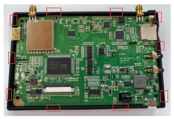
2.Insert the first buckle from this corner with a nail or tools.
