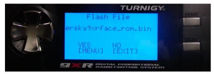
Long press MENU. The new firmware will be flashed to the transmitter, with a progress bar shown. Wait until you see "Flashing complete" in a few seconds. Turn OFF the transmitter.
