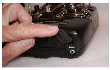
Your new 9XR Pro may come with a card already installed containing files such as firmware, voice clips, manuals, etc. It's a good idea to make a backup of the contents of this card on your computer.
