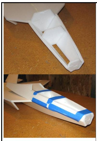
**11.**Use a sanding block to lightly sand the top of the lower forward fuselage until it is flat and even. Then glue on the upper half of each of the three forward fuselage bulkheads.
