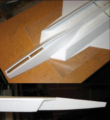
5. Glue the forward fuselage lower assembly in place on the front of the wing. Make sure the aft end of the forward fuselage mates with the forward edge of the centerline support piece. Also make sure the curvature is smooth as the angled forward fuselage sides twist to meet the vertical centerline support. Some trimming and additional heat-forming will likely be required to get a smooth curve here.
