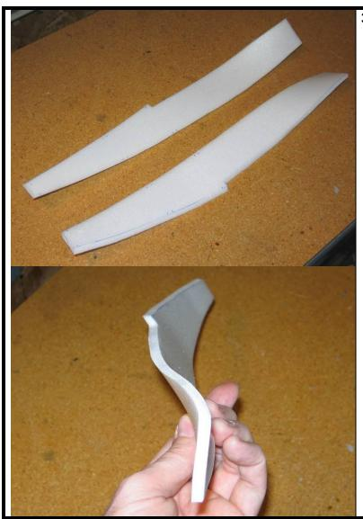
**3.** Cut bevels on the edges of the forward fuselage pieces as indicated on the plans. Be sure to make mirror-image left- and right-side pieces.
