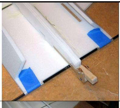
**7.** Glue the completed motor mount into the slot in the aft fuselage centerline support, aligning it to a zero-zero thrust line (no left/right or up/down thrust angle). Use 5 minute epoxy.
