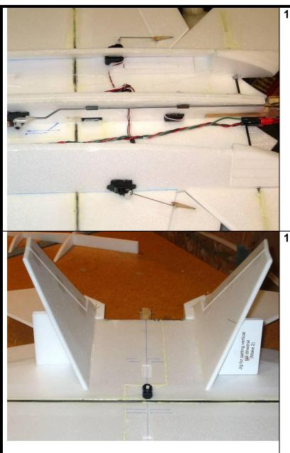
**15.**Next install the flaperons. Cut a 45 degree bevel in the leading edge of the flaperons using a ruler and a hobby knife, and then sand the trailing edges to a tapered shape. Then hinge the flaperons with strips of 3M Gift tape top and bottom. Trim as necessary to provide a small and parallel gap from the leading edge of the stabilators.
