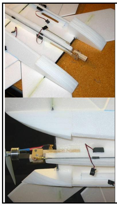
14. Laminate the tail boom pieces together using 3M 77 adhesive. Then glue the tail boom blocks to the aft fuselage with epoxy. Note that you'll need to carve out a small channel in the top of the tail boom blocks first to clear the aluminum stabilator pivot tubes. Make sure the tail boom blocks fit tight against the stab pivot tubes, since they provide significant extra strength to the stabilator pivots.
