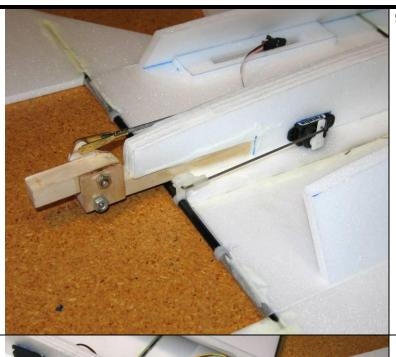
**9.** Install the stabilator servo into the slot in the fuselage centerline support (thick CA can be used to hold the servo in place). Make and install a music wire pushrod to the stab control horn. Once everything is properly aligned, glue the stab control horn into place using thin CA.
