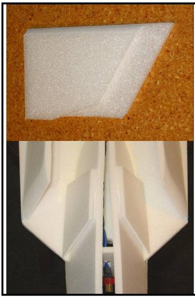
**21.** Laminate the inlet diverter piece and inlet side piece together as shown in the top photo at left, using 3M 77 adhesive. Make two assemblies. Then glue the assemblies at the front of the inlets as shown in the bottom photo.
