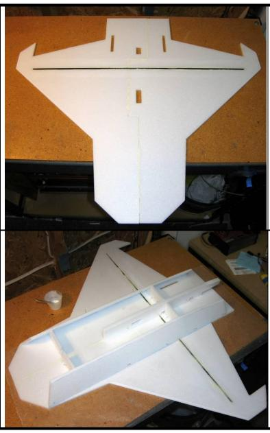
1. Begin with the wing. Cut a slot to fit the carbon wing spar and use 30 minute epoxy to spar into place. Mixing some microballons into the epoxy is recommended to reduce weight and help the glue fill gaps better (you can also use ProBond). Place wax paper and some heavy books on top of the wing to hold it perfectly flat as the glue cures.
