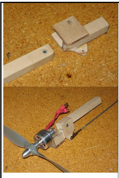
**6.** Next assemble the thrust vectoring motor mount. This step is optional—you may choose to install a straight motor stick if you don't want thrust vectoring.
