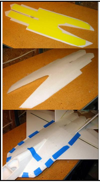
**19.** Next shape and install the aft fuselage top piece. This is perhaps the most challenging aspect of building this model, so take your time. There are many ways to form the curvature required, but I'll describe the particular method I used.
