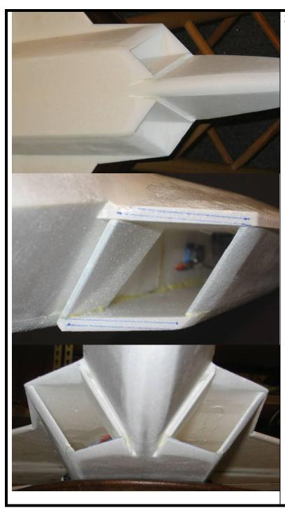
**23.** Now shape the inlets and aft fuselage. Begin by cutting slots in the aft fuselage bottom piece to provide exits for the inlet diverters (see top photo at left). Use a hobby knife inserted between the diverter pieces to cut the slot, and then trim with sandpaper.
