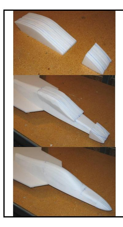
**13.** Laminate all of the nosecone and canopy pieces together using 3M 77 adhesive. Then glue the nosecone block to the front of the fuselage.
