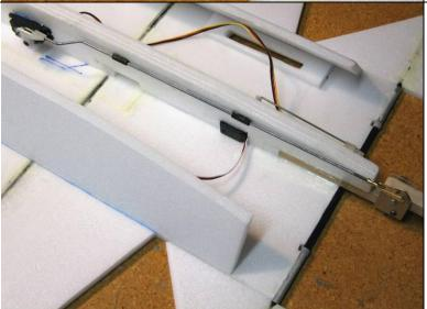
**10.** Next install the thrust vectoring servo and pushrod. A strong (40+ oz/in torque) metal-geared servo is required since a plastic-geared servo could get stripped if the prop hits the ground during landings. The prototype used a Hitec HS-85MG servo, which worked very well. Install the servo in the slot in the fuselage centerline support, securing it with CA.
