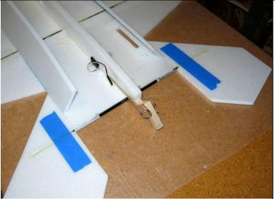
**8.** Sand the leading edge of the stabilators to a well-rounded shape, and the trailing to a tapered shape. Apply a strip of 3M Gift tape to the leading edge for smoothness and durability.
