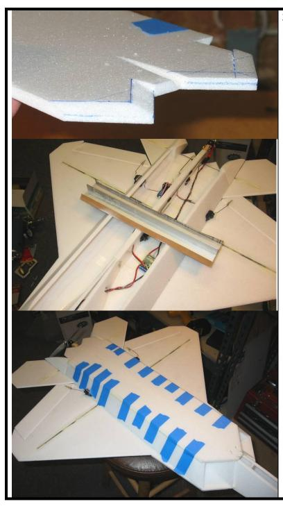
22. Next make and install the aft fuselage bottom piece. Begin by cutting the bevels in the sides as shown on the plans. Also cut bevels in the exhaust nozzles as shown in the top photo at left. You'll also need to carve a small notch in the center between the exhaust nozzles to provide clearance for the thrust vectoring pushrod and clevis (test fit the part to determine how much clearance is required).
