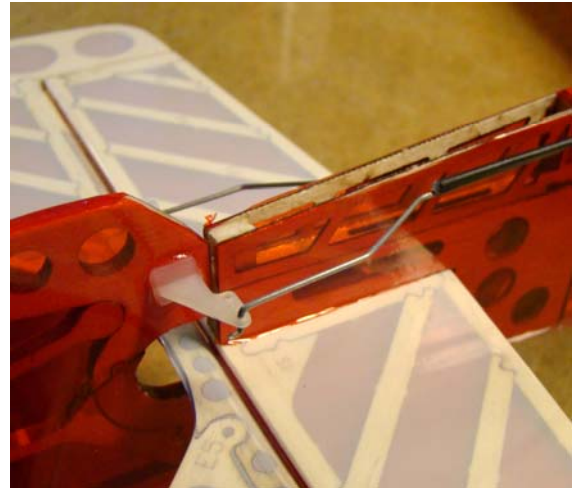
Fig 47: Install rudder pushrod using the same procedure.
