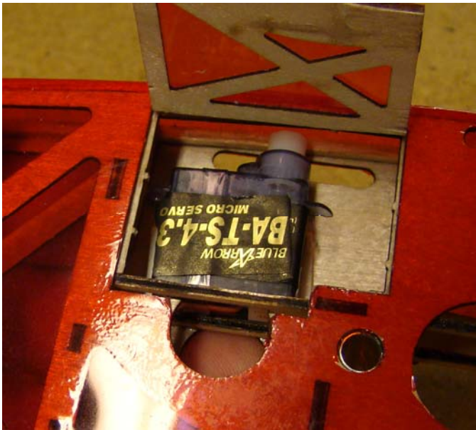
Fig 41: Position your servo. Center servo arm on servo arm slot located on the opposite side of your servo hatch. Hold servo up so tape does not stick. When servo is in position press down on servo while holding the outside wall of the fuselage to ensure you do not break the fuselage. Install second servo in the same manner.
