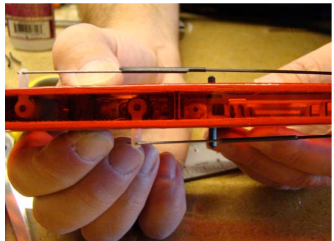
Fig 44: Assemble as shown with 1” overhang on shrink tubing. Pull back. Apply CA glue then apply heat to the shrink tubing. Repeat for other side, with longer push rod. *Note* Push rod guides are still NOT glued. Take push rods and set them aside.
