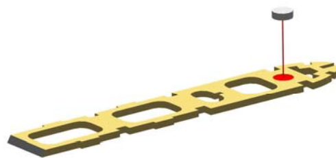
Fig 6: Bevel bottom edge of F4 45° and glue magnet in place.
