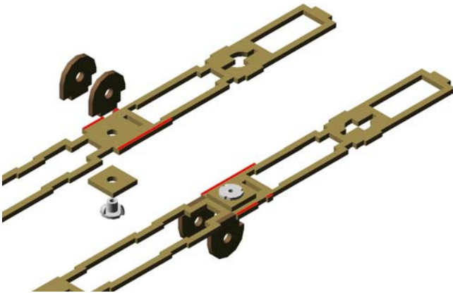
Fig 3: Glue the square reinforcement block to the bottom of the main fuselage former. Install 2-56 blind nut. Note that the main fuselage former is marked side A and side B to match the fuselage sides. Glue the two F11 pieces into place.
