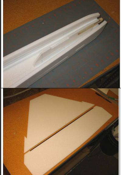
8. Glue the hardwood motor stick into the foam motor mount with 5 minute epoxy and let it cure. Then glue the motor mount into the aft fuselage (5 min epoxy recommended), making sure it is aligned with the centerline drawn on the fuselage bottom.
