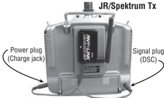
**!** **WARNING! Do NOT turn the JR or Spektrum Tx power switch to the ON position at any time!** This will cause AnyLink to stop sending signal to the Tactic Rx and result in a loss of control of the model! The JR/Spektrum Tx power switch should ALWAYS remain in the OFF position when controlling a model with AnyLink.
