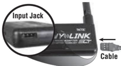
**Futaba transmitters:** For computer radios which offer the option to transmit a signal when Tx power is turned ON, make sure “YES” is selected. Then turn the Tx power switch OFF. Connect the cable’s square trainer plug to the Tx trainer jack and skip to the next section.
