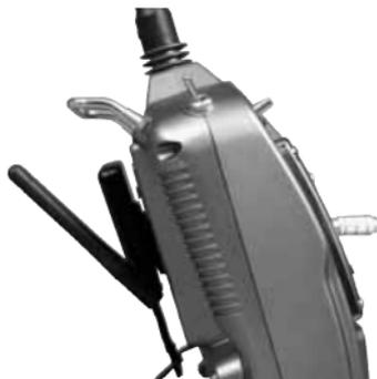
Mount AnyLink high on the rear of the Tx, and extend its antenna to point upwards from the top of the Tx as much as possible. Rotate the antenna as shown above. Two strips of hard locking fasteners are included for attaching AnyLink to the rear of the host Tx.
