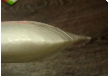
Put the wing under the load so spar and trailing edge stick along the entire length, and the wing had no twist.
