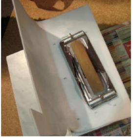
In one go glue the ribs and spar to one side of the wing shell. And while the glue is fresh glue another side and wrap the wing shell. Then you have to hold the wing for some time to let it dry.
