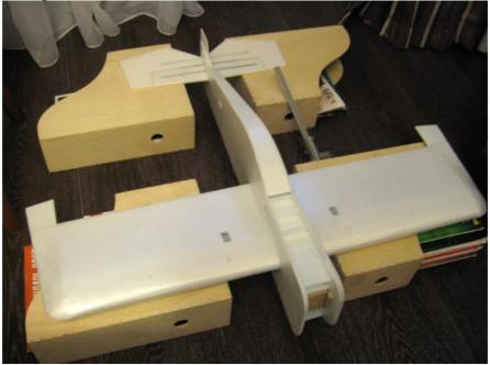
Make undercarriage support from balsa wood. Glue undercarriage with the help of threads and CA.
