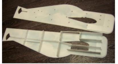
Glue in the plywood motor frame, the fin and glue the fuselage halves together. Place the fuselage under the load, make sure the halves did not shift.
