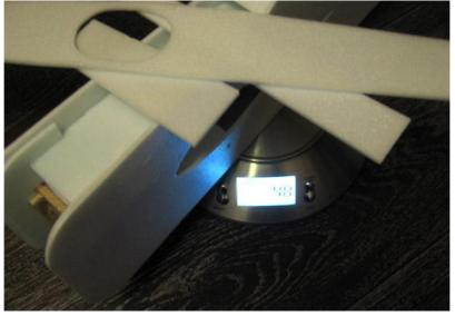
While fuselage and wing are drying, let's make the horizontal stabilizer and the control surfaces. If you want to build a light aircraft, the stabilizer should be single-layered (3mm thick). If you want the aircraft to be under 370 gr., control surfaces can be dual-layered (6mm thick). Thicker stabilizers will allow greater precision in all maneuvers. (The photo shows double control surfaces and stabilizer). The ailerons can also be dual-layered, but the control is less affected.
