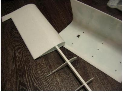
Cut the edges on wing tips at 30-45 degrees. Glue the edge and fix it with the adhesive tape to make it stick together.
