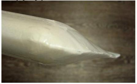
This can be easily fixed with adhesive tape and an iron. The trick is to select the temperature, so the scotch-tape can stretch and depron does not melt.
