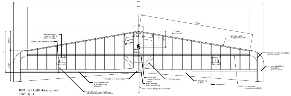
Lite Ply ribs epoxied to spar, No rib caps
