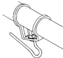
120-100 Jib Swivel with Ball Race Adjustable for Round 10mm dia. Boom
