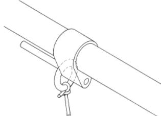
46-100 Boom Band with Pin - Fits 10mm dia. Round Tube. Used in conjunction with 46b as Jib swivel (does not include ring 46b **BUY EXTRA: US\$ 3.92**)
