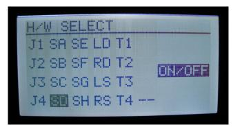
**STEP 3**: In this example switch **SD** is selected to change Dual Rates and Exponential Settings.
