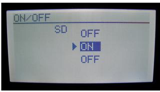
**STEP 4**: Now you should see the screen on the left. Here you actually set which of the three positions of switch **SD** turns Dual Rate and Exponential **ON** or **OFF**. In this case, the center position of switch **SD** is the **ON** position.
