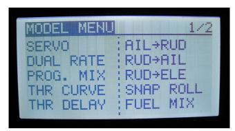
**STEP 1**: Select **MODEL MENU** by tapping **MDL** on the right hand side of the Sensor Touch "scroll wheel" twice.
