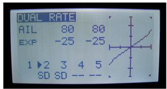
STEP 2: Scroll through the **DUAL RATE** screen. Pointing the cursor to the item to be changed, tap **RTN** on the scroll wheel. The item becomes a hollow rectangle. Moving over the scroll wheel will present the options (for example **AIL** becomes **ELE**, **RUD** and **THR**).
