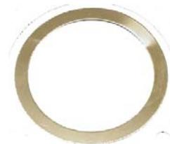
If you do not use the extra shim the engine will not run smooth and you will get symptoms like if you are using a glowplug which is too hot. But no plug is available which is cold enough to compensate the pre-ignition. You have to use the extra shim.
