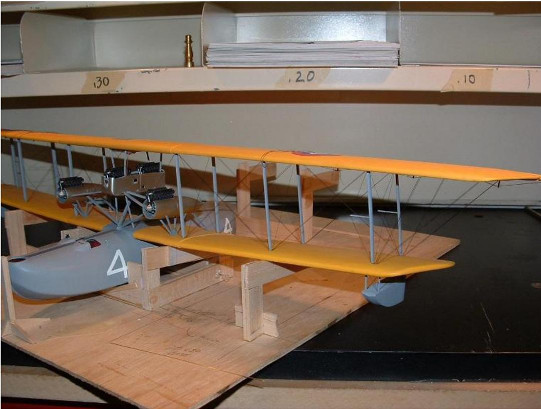
*Lycra was used for Wing Bay and Control Line rigging, Monofilament was used for the Tail Booms for strength and to hold it all in place.*
