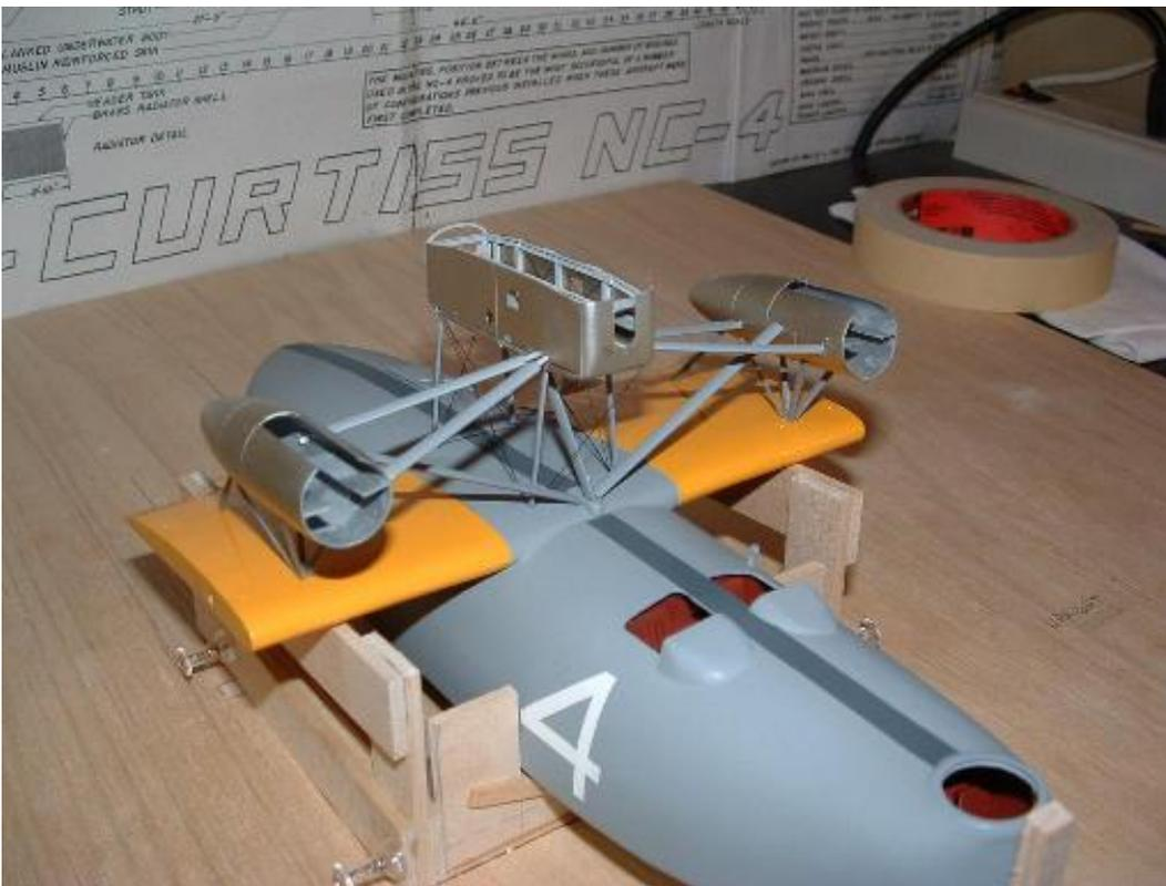
*Nacelles after being painted, and the forest of struts cut to fit. Cradle for Assembly Jig helps hold everything in constant alignment to keep things square and even.*
