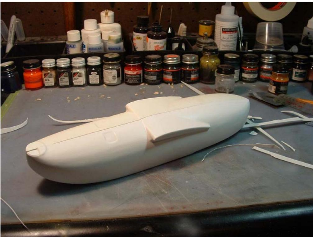
*Hull after vacu-forming. The basswood master was cut in half at the Cockpit Bulkhead and left in the rear portion of the hull for strength. This allowed for brass tube sockets for the lower wings to plug into. (And to prevent me from being loony enough to build a second one)*
