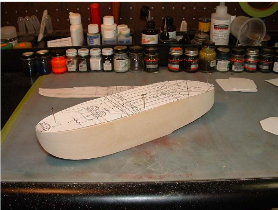
*Hull begins life as paper templates pinned to the wood block and band sawed to shape, then a small block plane was used to rough carve the hull to close to final shape.*
