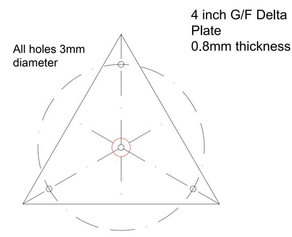
Do not drill the 9.5mm hole (Red Line) until the Motor mount has been test fitted and its mounting holes drilled
