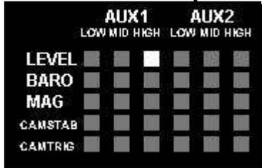
Depending on your configuration, you can easily activate/deactivate options via 2 switches on your RC TX. The 2 switches correspond to (AUX1), typically RX ch5 and, RX channel 6 (AUX2).
