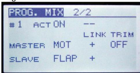
Now set up a new Program Mix. On screen 2/2 change INH to ACT. Set the MASTER to MOTOR and change its LINK from OFF to +. This will allow the master to access its related speed control function.
