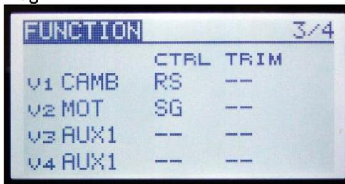
As the Motor Function is not going to operate a servo or ESC directly, it can be assigned to a virtual channel to avoid tying up an active channel. In the FUNCTION MENU assign MOTOR to any of the free virtual channels on screen 3/4. The throttle stick will be assigned by default as the control so change this to a suitable three-position switch for controlling the flaps. SG is used in the example (see Diagram 2).
