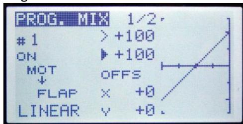
Check the servo monitor and the flaps should respond to the switch with reduced speed.
