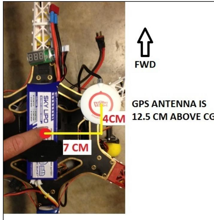
NOTICE THE GPS ANTENNA IS FORWARD AND RIGHT OF THE C.G. THEREFORE BOTH X AND Y VALUES SHOULD BE POSITIVE NUMBERS
