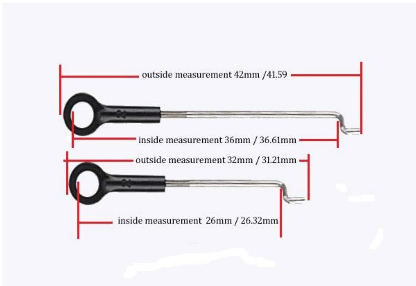
These lengths are base line measurements only. With these lengths, the helicopter should hover or take off with a drift backwards and to the slightly to the right.
