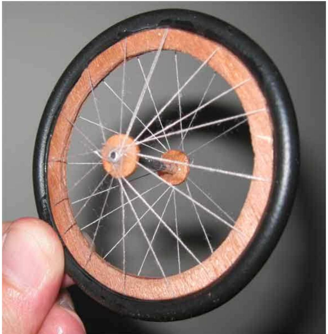
Build your own thread [RC plane plan](#) spoke wheels - no special tools required
