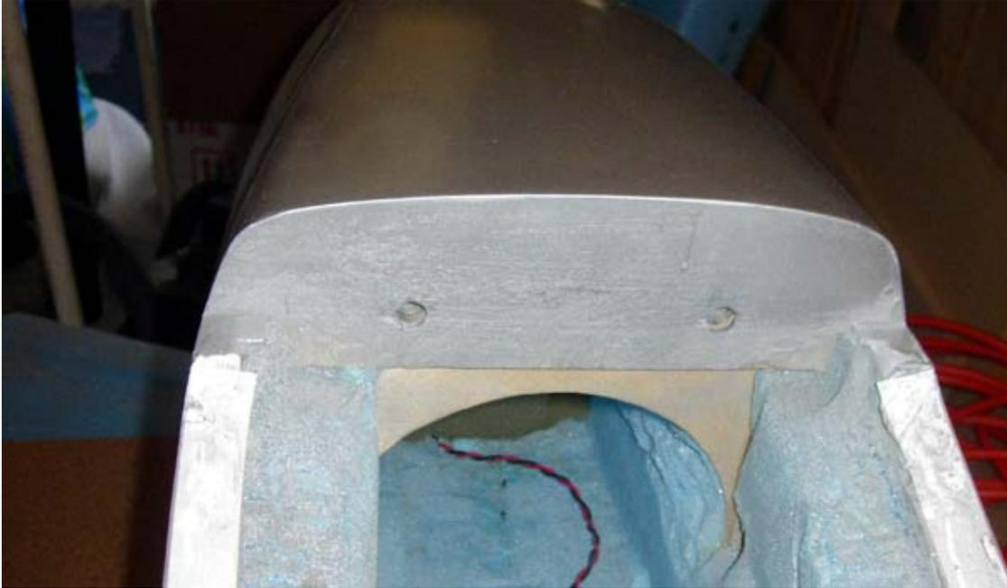
26. Apply a 1/16" thick by 3/4" wide plywood wing saddle plate to each side of the wing saddle and epoxy in place by bolting the wing on to hold in place. It may be necessary to trim the fiberglass and foam back slightly to make room for the plywood plate.
