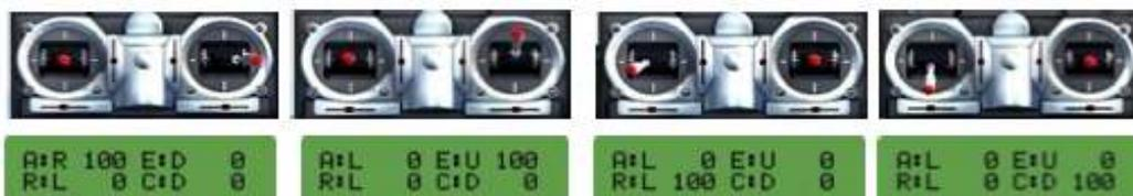
Examples of stick travel where the value should read 100. Also note the "L", "R", "U" & "D". Press the DOWN/DATA- key to select the second page, showing the transmitter channel gain signal and the gyro parameter set currently in use:
