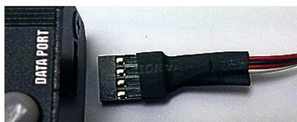
Note the correct orientation of the data cable plug
