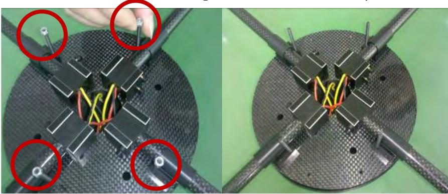
b. Pull out bar (LG), make the Slot match the cross beam and screws on Base.
