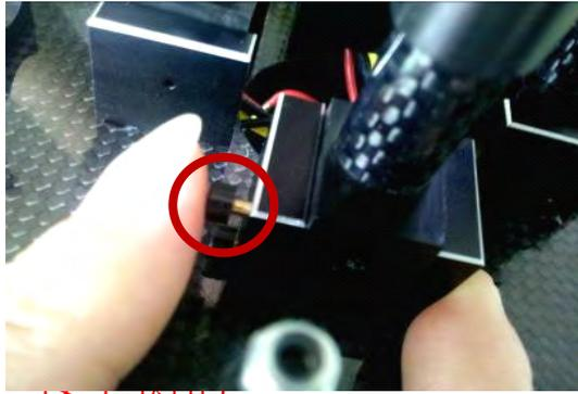
b. Pull out cross beams, press on fixing pad, you may hear clear "click". It says cross beam unfolding condition is locked.
