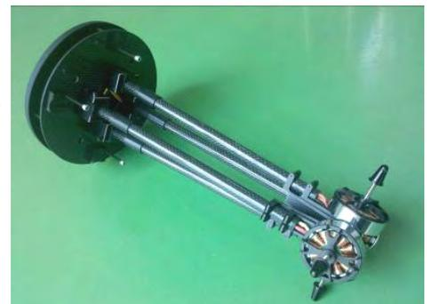
a. Press relative locking keys, you will open 4 P4 arm beams.
