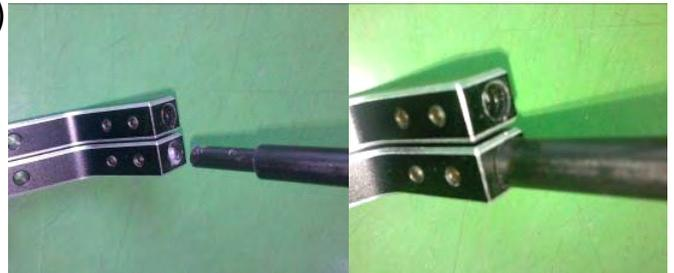
b. Lock two Hex screws at the inner side of the arm tightly, be carefully and do not break glass fiber pole.
