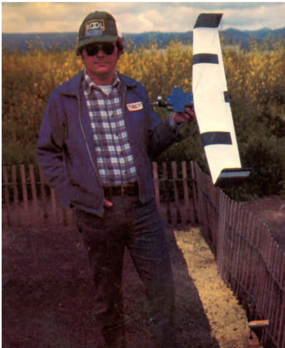
Dave Pastor displays his  $\frac{1}{2}$ A RC cutie. He used a sliding servo tray for operating the strip elevens but notes that mechanical mixers will work just as well. Construction is super simple.
