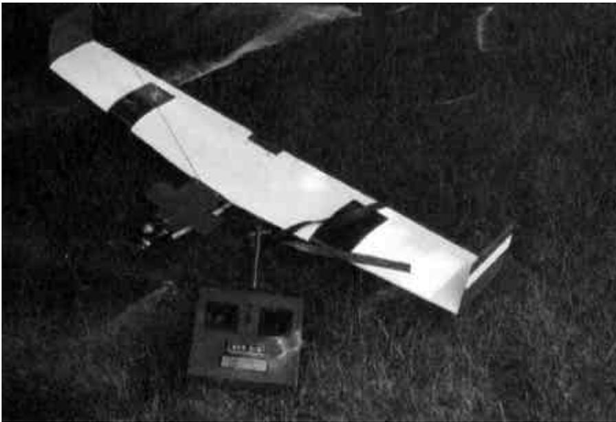
All you need for this one is a two-channel radio setup. It hand launches easily, and if you mount the prop horizontally as it begins to come up on compression, it will help save the prop on landings.
