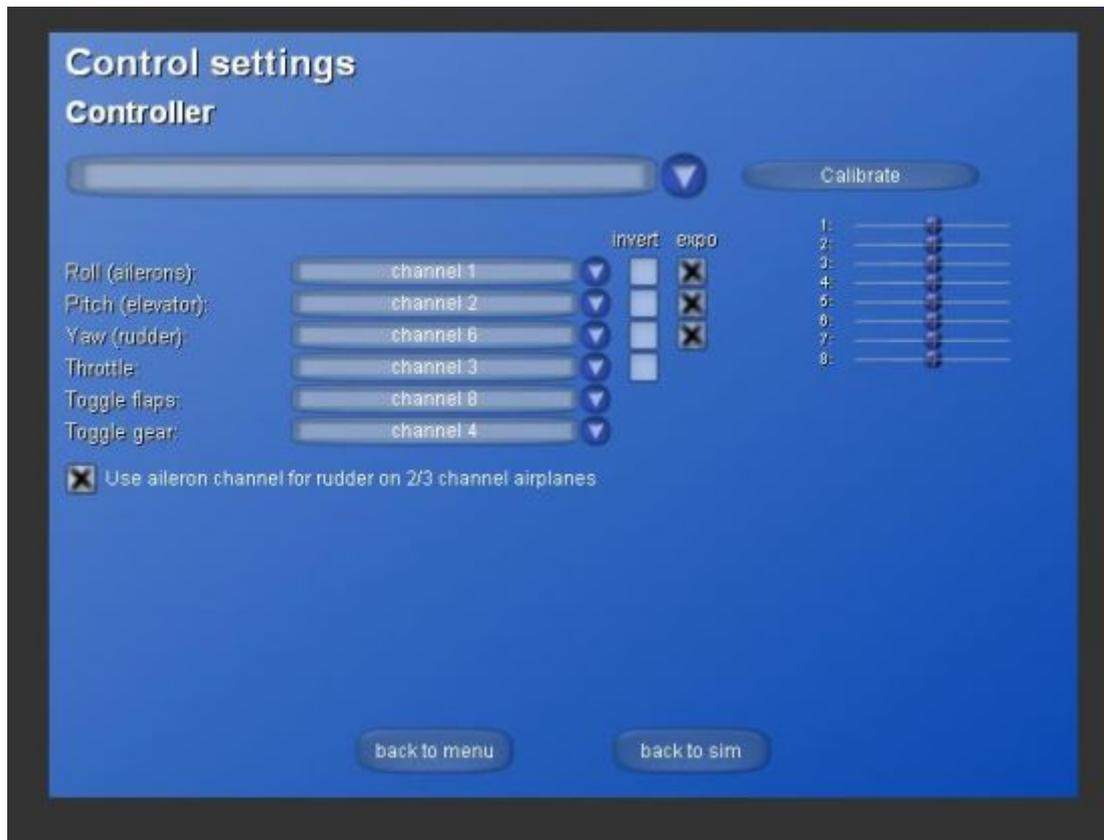
Note: Mode 1 & 2 are output to the same channels as seen by Receivers, Slave TX (Buddy/Trainer) and Simulators so TX mode does not matter.
