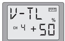
6. Once this mix has been activated, move the servos to their full extremes to make certain they are not overdriving the controls. If necessary, adjust the linkages to achieve the correct control throws.
