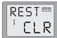
3. Push **DATA INPUT** upward or downward for about 2 seconds to clear and reset the memory. "**CLR**" blinks first, and then it stops blinking with a sound. Now the model data is reset to the initial setting that is the default value set at the factory.
