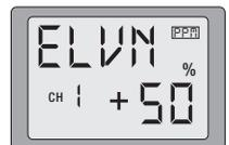
5. Next you set the right wing to channel 2 (elevator) setting. Press the SELECT key to display the “CH2” and flashing “%” sign. Use the DATA INPUT lever to set the percentage of rudder travel rate from -100% to +100%
