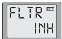
2. If "INH" is blinking, push DATA INPUT lever upward. Then you will see that the blinking "INH" changes to "ON". Your flap trim is now turned on.
