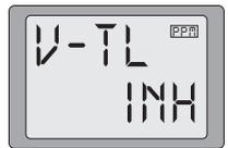
You cannot set "V-tail" mixing when "Elevon" mixing has already been set. In order to enable "V-tail" mixing, you first need to cancel "Elevon" mixing. However, it is allowed to use "V-Tail" and "Flaperon" mixing simultaneously.
