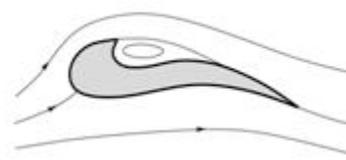
Figure 2. Airfoil with a trapped vortex
