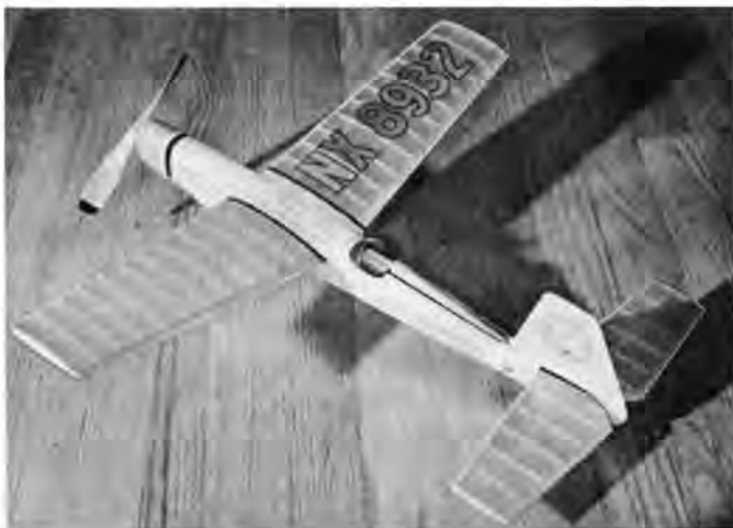
The wing is permanently attached to the fuselage and faired in. The cockpit is an inspection hatch for the rubber.
