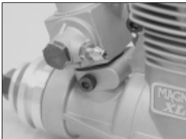
of the carburetor into the crankcase, being careful to keep the carburetor perpendicular to the front of the engine. Using your thumb, push down firmly on the carburetor so that the base of the carburetor sets completely into the crankcase. An o-ring is installed on the carburetor throat to seal the joint. While holding the carburetor firmly
