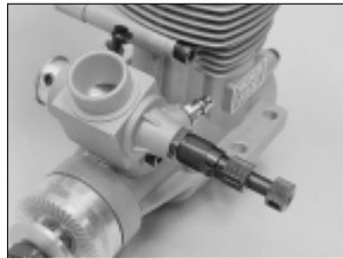
Using an adjustable wrench, carefully loosen and remove the plug from the side of the carburetor. Carefully loosen and remove the needle valve assembly (including the clear gaskets) from the rear
