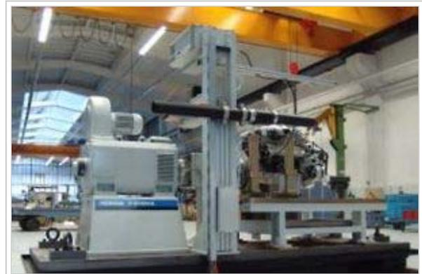
HORIBA engine dynamometer TITAN
