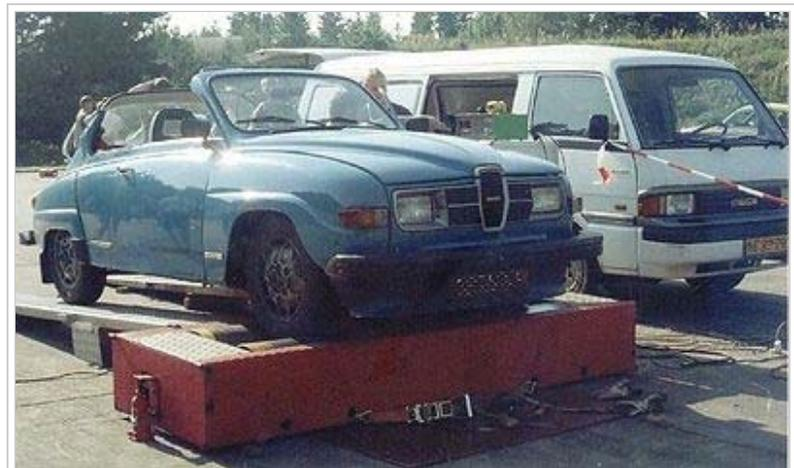
Saab 96 on chassis dynamometer
