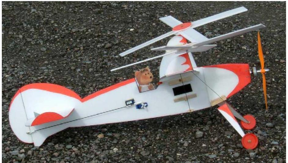
*The twin rotor design offers a number of advantages compared to a single rotor. Easy to build, easy to repair, with no complicated linkages to the rotor head.*
