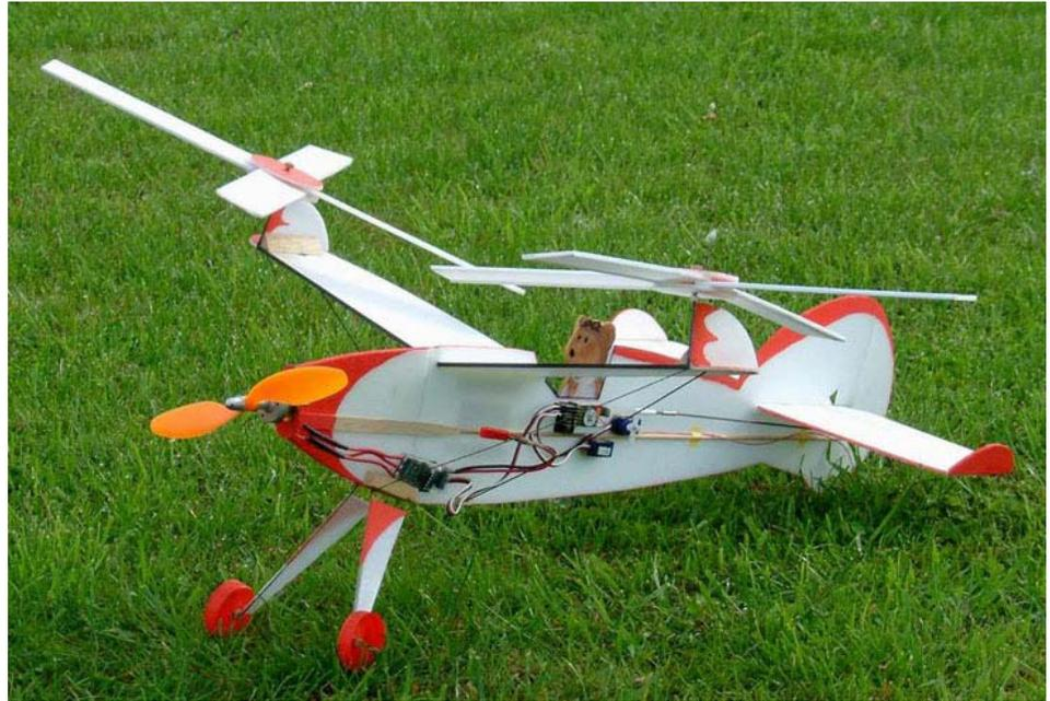
*A slave to 3mm Depron, Twirl's flat plate profile goes a long way in providing a light all-up weight of around 7oz (200g).*
