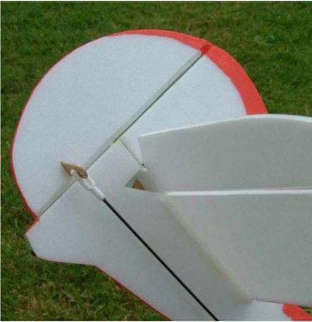
*Rudder and elevator leading edges are chamfered at 45° prior to being top-hinged.*
